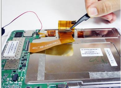
On the metal plate inside of the device, there is a ribbon cable in a loop. Flip the white tab and pull the cable out.
