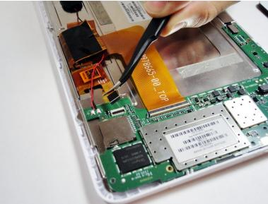
Remove the smaller ribbon cable by gently flipping the black latch and pulling it out with tweezers.
