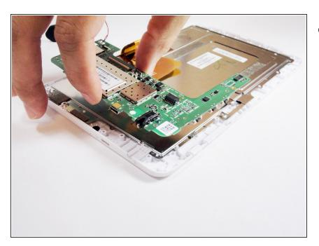
Carefully lift the motherboard directly up.
