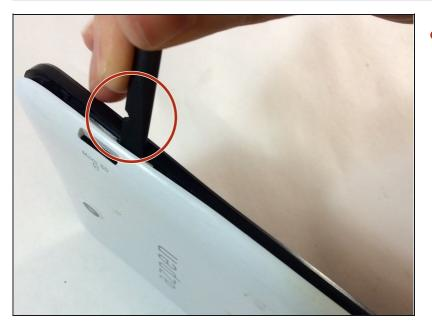
Use the plastic opening tool or black spudger tool to lift the back panel off the tablet.
