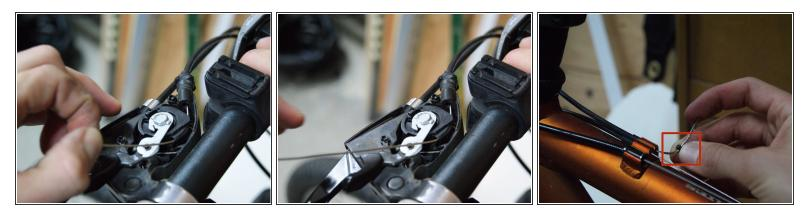
• Pull on the shifter end of the cable to pull the cable free of the bike, through the shifter and all the housings.
