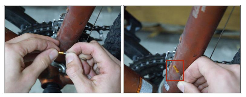
Place the crimp on the cut end of the cable, making sure to get any loose strands within the crimp as well.
