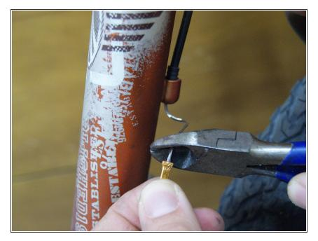
If the cable is not already cut, cut any excessively frayed ends or crimps off the end by the derailleur so the cable can easily be pulled back through the housings.
