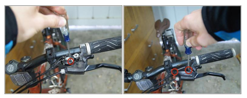
• Reassemble the shifter, putting back the indicator, the case, and their corresponding screws
