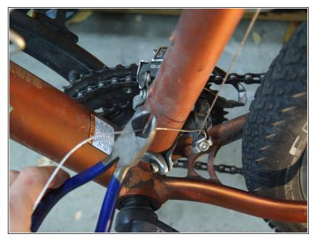
Once the derailleur is in the correct position, cut the cable to length, leaving 2 to 3 inches to allow for later adjustment if needed.
