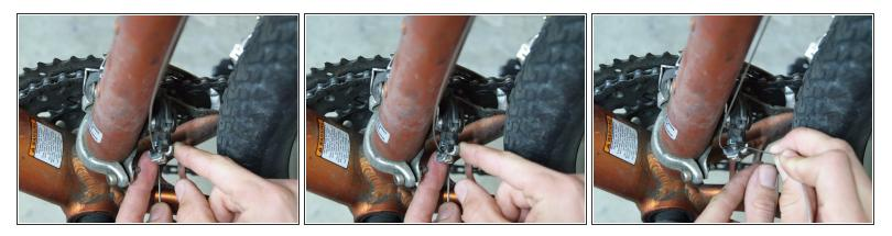
• Run the end of the cable around the tightening Allen bolt, between the silver holding plate and the derailleur body.
