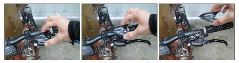
• Remove the shifter casing (the top) from the shifter body.
