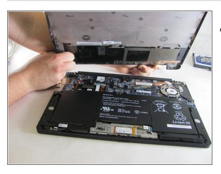
Lift off back cover to access inner components of computer.
