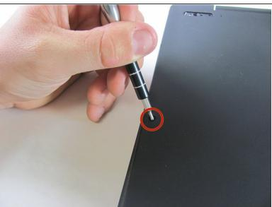
Starting with the laptop top-down, locate and remove the twelve 1mm Phillips #0 screws securing the back cover to the main body of the computer.
