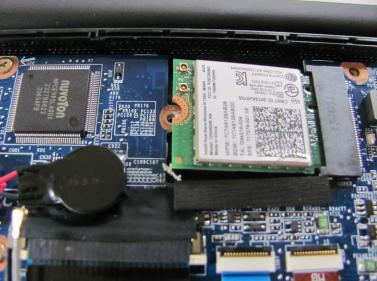
Locate and remove the single 1mm Phillips #0 screw that is securing the wireless card to the motherboard.
