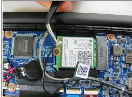
Use a pair of tweezers to gently disconnect the two antenna cables.
