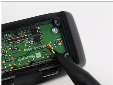
Using the spudger or the tweezers, gently detach the golden connector from the motherboard.
