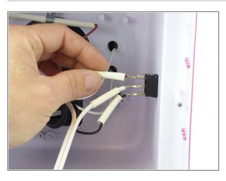
Pull back the insulation sleeves to expose the connector heads.
