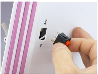
Remove the switch from the device.
