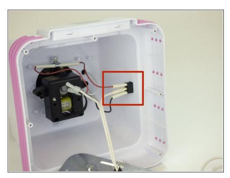
Locate the switch/wire assembly inside the device.
