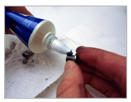
Now that the chainring bolts are clean, apply a pea-sized amount of grease to each bolt.
