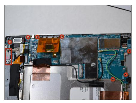
Use a Phillips #000 screwdriver to remove the screws around the perimeter of the motherboard.
