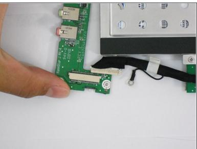
Disconnect the I/O board from the motherboard.
