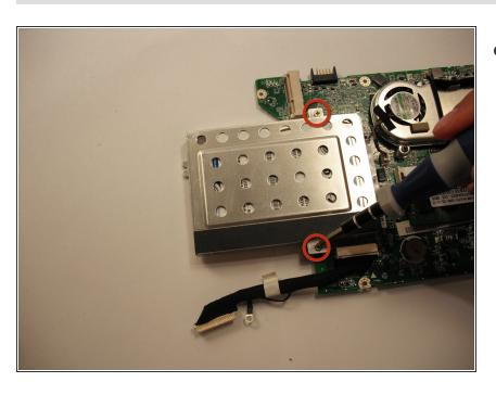
Remove the two 4.7 mm Phillips #0 screws that hold down the hard drive.
