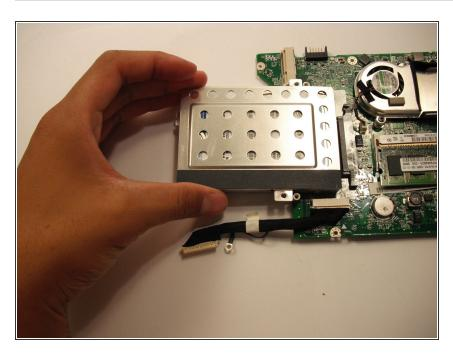
Pull the hard drive straight out from the motherboard.
