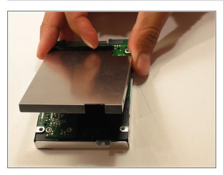
Remove the upper and lower casing from the hard drive.
