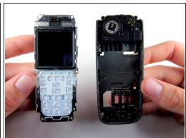
Lift the circuit board out of the back cover.
