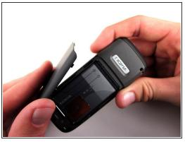
Place your thumb on the middle of the back cover and push it toward the bottom of the phone to slide the cover off.
