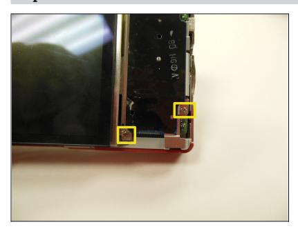
Remove the two 3.85 mm screws on the bottom right of the camera, as indicated.
