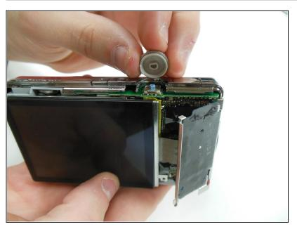
Remove dial button located on top of camera, by gently pulling up.
