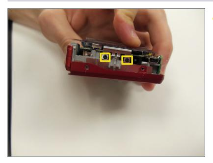
On the right side of the camera, locate and remove the two 3.25 mm screws as highlighted.
