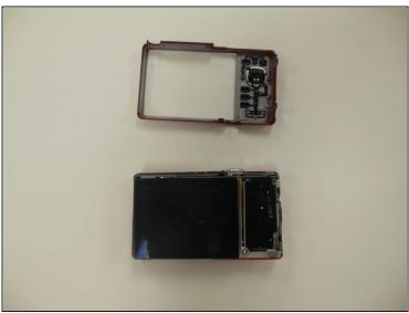
• Using both hands, carefully pull the frame apart from the camera.
