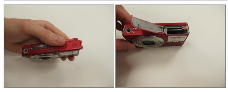
• First, press in and slide forward the battery latch as indicated by the arrow.
