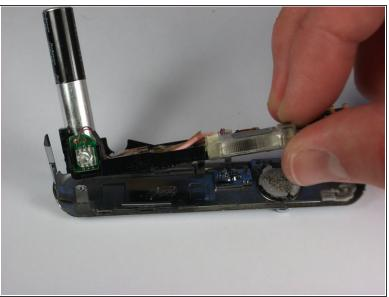
After, releasing all the components, gently remove the flash assembly from the casing.
