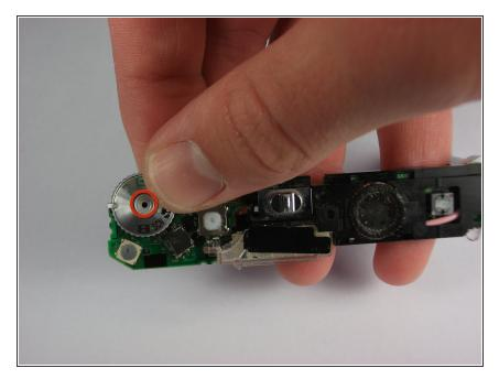
Remove the 1.2 mm screw from the settings wheel.
