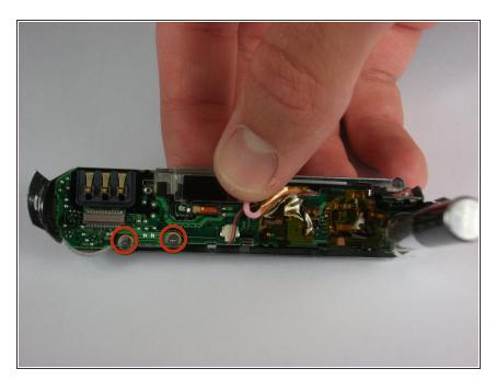
Remove the two 3mm screws.
