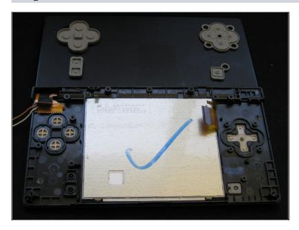
Reach under the front of the device, and push the bottom screen towards you, out of the frame.
