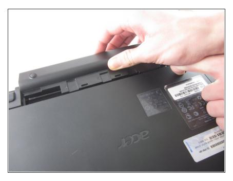
With the switch slid, pull out the battery.
