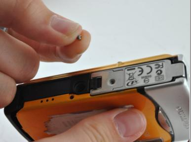
Using a PH00 Phillips Screwdriver, unscrew the one screw located on the latch.
