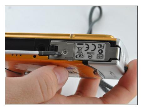
Locate the battery compartment on the bottom panel of the camera.
