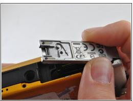
• Find the arrows on the compartment, remove the small black plastic piece, and release the latch.
