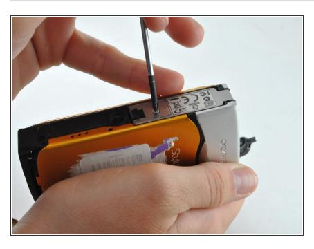
Place the metal cover back over the closed latch, and screw the screw back in.
