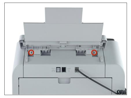
Remove the two 15 mm Phillips #1 screws securing the ADF at the rear of the fax machine.
