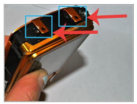
You will need to remove the front panel in order to access the lens. Lift the latches on the side of the front panel to remove it entirely, pulling gently in an upward motion.
