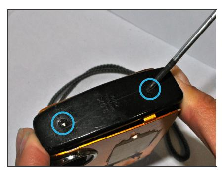
Unscrew the two small screws on the black side panel of the camera using a PH00 screwdriver. Remove the part.
