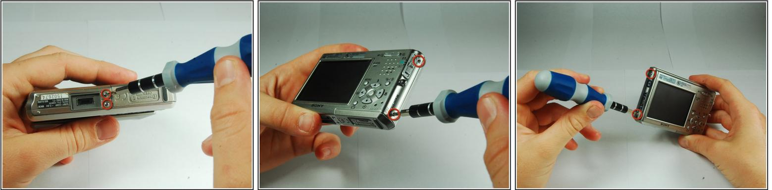
**i** There are two screws on the left and right sides of the camera, and two screws on the bottom.
