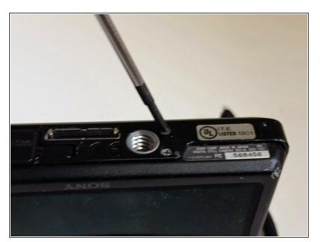
Use the Phillips #00 screwdriver to remove the 4mm length screws.
