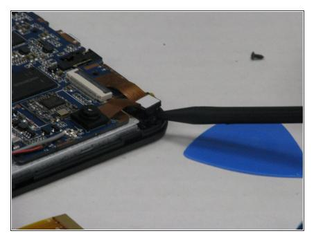
Use the spudger in the top corner of the tablet and lift the camera up.
