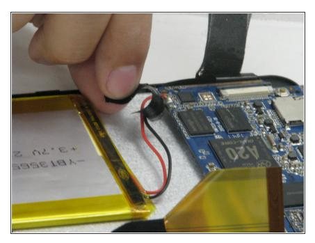
Lift the tape over the wires that are holding them to the tablet insulation.
