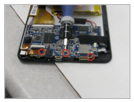
In order to unseat the motherboard, use the Phillips PH00 screw driver bit to remove the three 1.2mm x 3mm screws.
