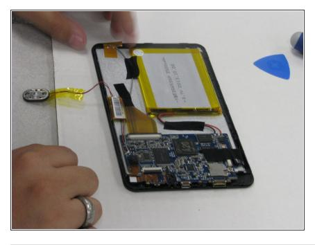
Remove the speaker unit from the tablet and set aside.
