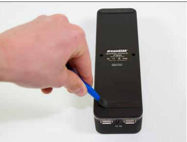
Remove the rubber foot pads on the bottom of the device using a plastic opening tool.
