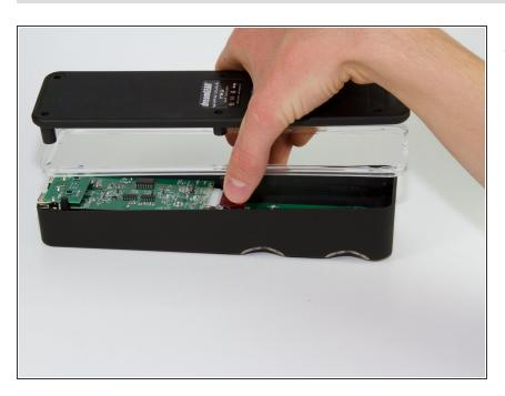
Gently remove the bottom of the device.
