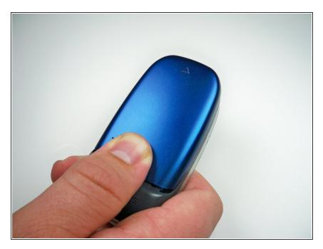
To remove the back cover, use your thumb to press down on the center of case and slide it off.
