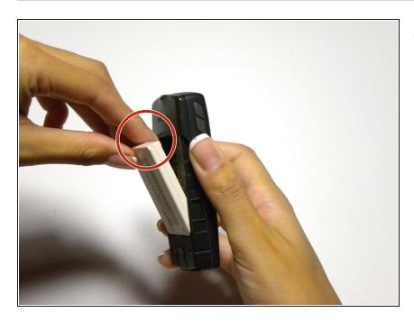
To remove the battery, push it down from the top and pull it out.
