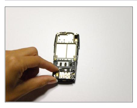
Grasp top and bottom of battery charger connector on the left side
