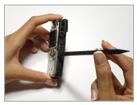
Insert spudger along edge of assembly and gently lift assembly away from case
