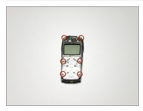
Remove the six screws using a T6 torx screwdriver.
