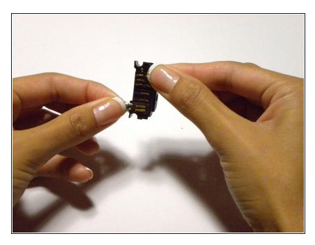
Grasp vibrator which protrudes from the battery charger connector
