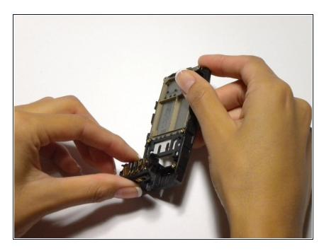
Lift out the battery charger connector
