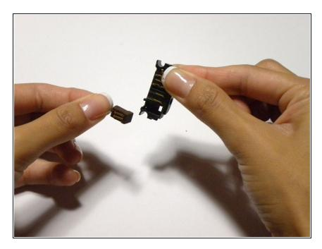
• Lift the vibrator out of the battery charger connector.
