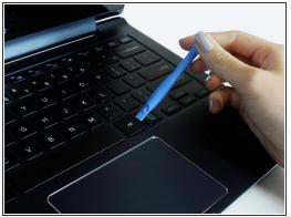
• Using a plastic opening tool, carefully push the thin tip under the key.
