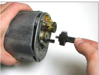
Remove the gear that is threaded onto the divider.
