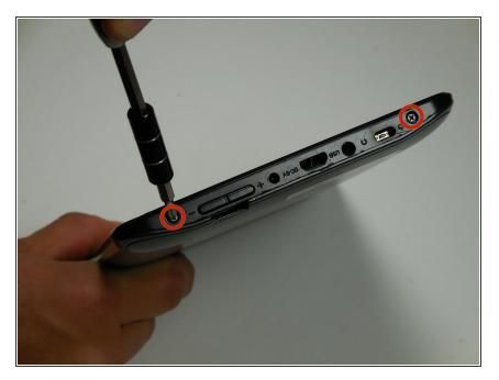
Remove the two 2cm screws on the bottom using the PH0 Phillips head screw driver.
