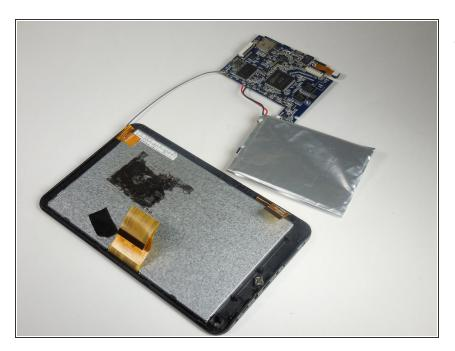
Remove motherboard and battery and set aside.
