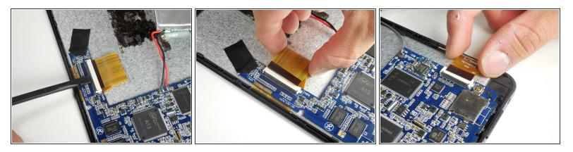
Disconnect the two larger of the three ZIF cables by prying open the flap with a plastic spudger and gently removing the cable.
