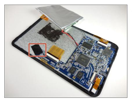
Peel off the black tape from the corner of the motherboard (indicated by the blue surface of the device)
