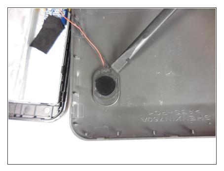
Disconnect speaker (which is attached by black and red wires) from back piece using plastic spudger.
