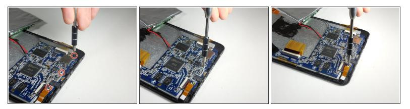
Use PH000 Phillips head screw driver to remove the three screws that connect the motherboard to the front panel.
