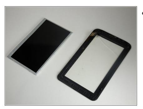
Replace broken screen and reverse steps to re-assemble device.
