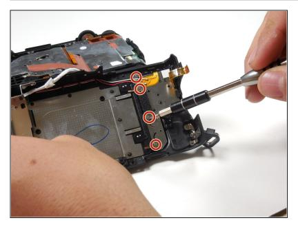
Remove the four 4.3 mm screws located on the far right metal plate. Use the Phillips #00 screwdriver.
