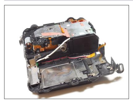
• Remove the back casing.
