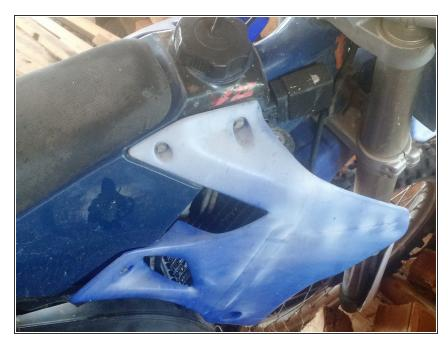
Next, you will need to check the patch after completely dry. Make sure there is no bubbles or edges where there could be another potential leak.
