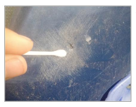
Once the hole is smooth. Apply fuel patch with q-tip over hole and the surrounding edges.
