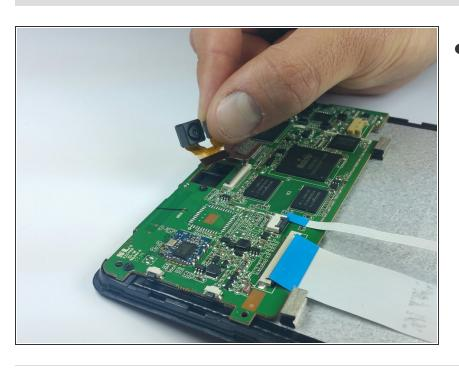
Pull both camera lenses out of the ribbon connector.
