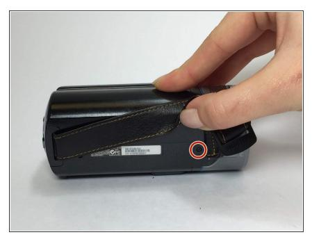
• Remove the 4 mm screw next to the buckle of the hand strap closest to the lens.
