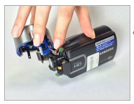
• Firmly grip and pull the front casing on the lens to remove it.
