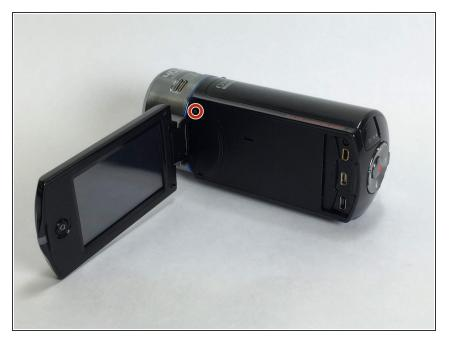
Open the LCD screen. Remove the 4 mm screw on the inside panel, located at top left corner.
