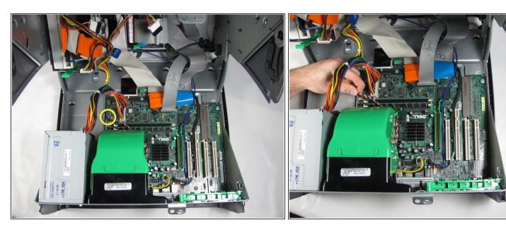
Disconnect the fan cable from the motherboard.
