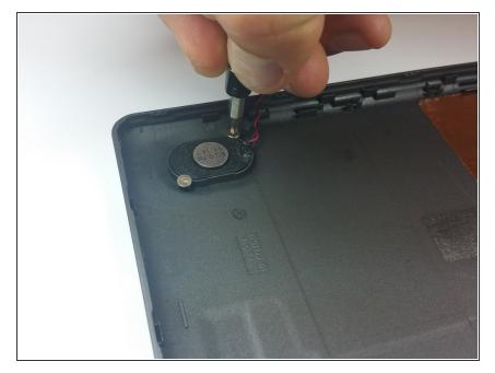
Remove the two 0.116 inch screws holding the speaker assembly in place.
