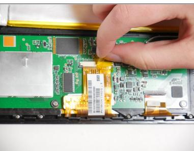
• Peel tape off of ribbon connectors. Starting at the power button, work clockwise around the tablet.
