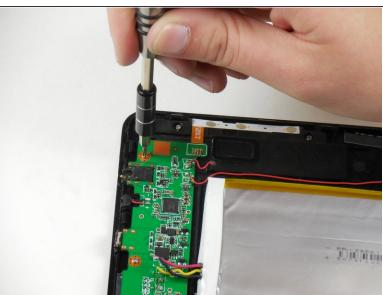
• Unscrew the thirteen 4.75mm screws around the perimeter of the tablet using a PH 00 screwdriver.
