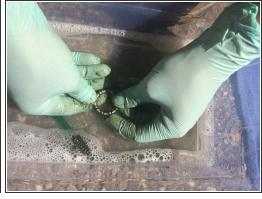
(i) When cleaning the bearings, spin the balls to help remove grit from inside.
