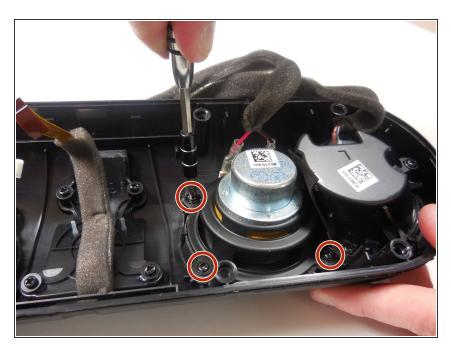
Using a Phillips #2 screwdriver, remove the 4 (8mm maxi-loc Phillips #2) screws holding the speaker to the case.
