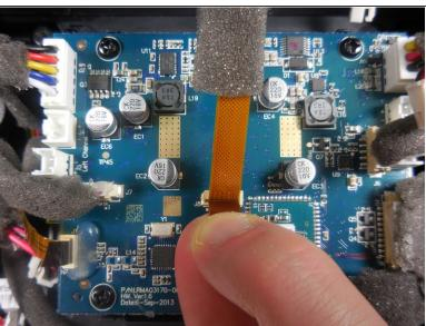
Gently pull on the plastic tab at the base of the ribbon cable to remove it from the motherboard.
