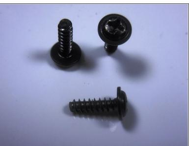
Using a Phillips #2 screwdriver, remove the 8 (10mm maxi-loc Phillips #2) screws that hold the casing together.
