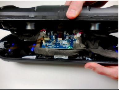
Pull apart the front casing from the back casing, slowly. Try to avoid any tension on any of the connected cables.
