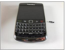
Use your T5 Torx screwdriver to remove the two black 5.57mm Torx head screws underneath the keyboard.
