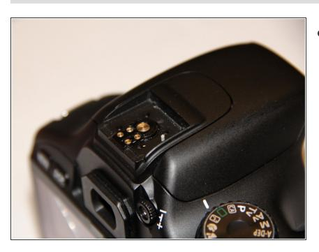
With the screws removed, the hot shoe can now be lifted out of place.
