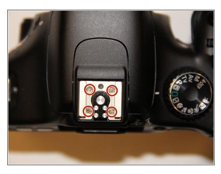
To remove the hot shoe, unscrew the 4 mounting screws holding it in place.
