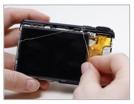
Remove the thin metal frame that runs along the top of the LCD screen.
