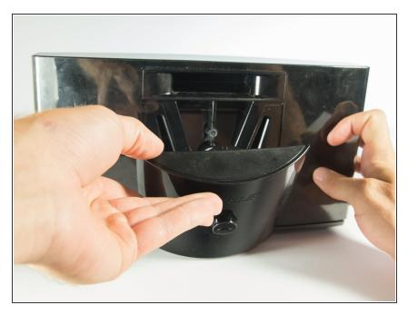
Carefully pull the battery away from the back of the system.
