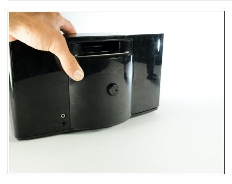
Push in the slotted knob and turn it clockwise until the slot is vertical.
