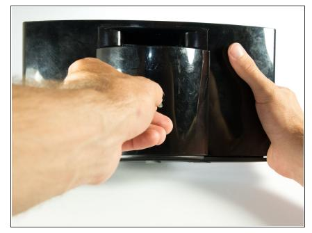
Using your thumbnail or a coin, push in the slotted knob on the battery and turn it counterclockwise to unlock the battery.
