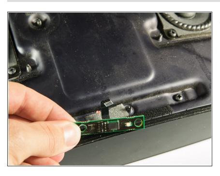
Using tweezers or your fingers, gently remove the ribbon cable connecting the IR sensor to the system.
