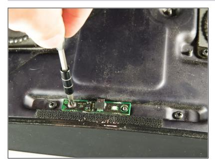
Using a T15 torx screwdriver, remove the 8mm screw holding the IR sensor to the speaker system.
