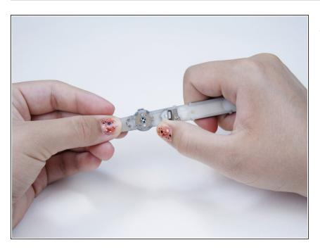
Flip the silver panel over. The power button is the smaller button covered by a metal backing.
