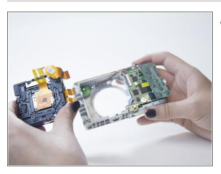
Pull the lens box up and out to remove it.
