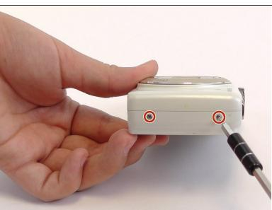
Remove the two 4mm screws from each side of the camera with a Phillips PH000 screwdriver.
