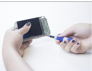
Using the Phillips PH000 screwdriver, remove the 4mm screw from the bottom left corner of the button plate located under the button membrane.
