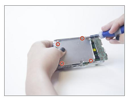
Remove the metal plate that was underneath the LCD screen by removing the four 4 mm screws with the Phillips PH000 screwdriver.
