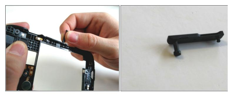
(i) The SD cover is held in place on the frame by a small tab.
