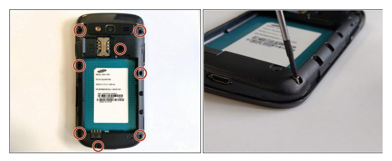
• Use a Phillips #00 screwdriver to remove the **eight** 4 mm screws from the device frame.
