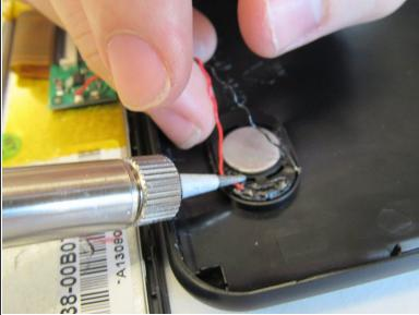
Solder the wires to the base of the speaker. The metal of the wire should be touching exposed metal on the speaker. Insure that the colors of the wires match the picture.
