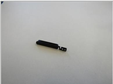
Align and place the new replacement button with positive and negative engravings facing outward into the volume space found in the cover.
