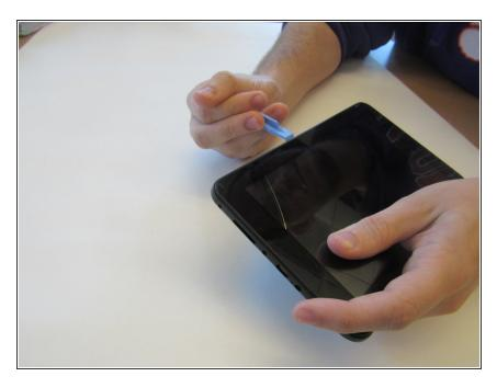
Separate the front and back covers using one of the plastic opening tools.
