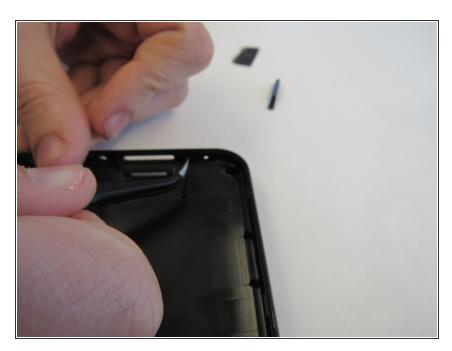
Dislodge the volume button from the upper right corner of the tablet's back cover using the tweezers
