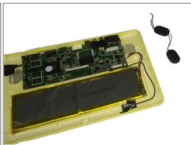
Pry the second speaker out of its holding place with a plastic opening tool or spudger.
