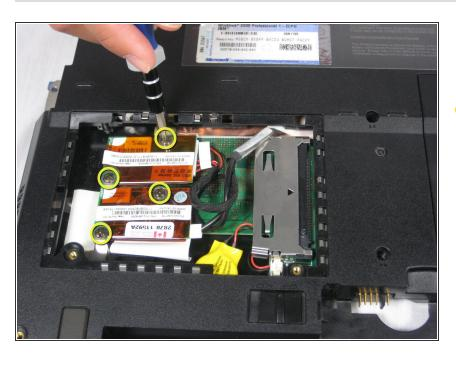
Remove the four 9.1mm screws attached to the ethernet and modem cards.
