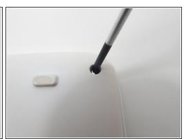
Remove four 5 mm Phillips #00 screws from each corner of the tablet.
