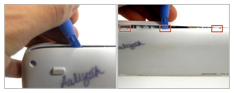
• Place the iFixit opening tool in the notches between the cases and pull the covers apart.
