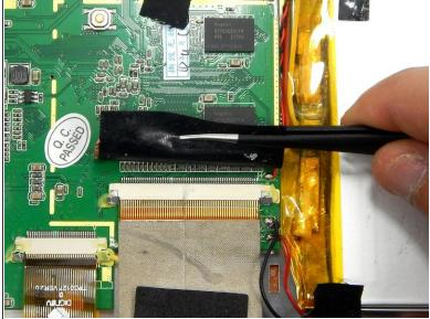
Peel the copper tape covering the ribbon connector with a set of tweezers.
